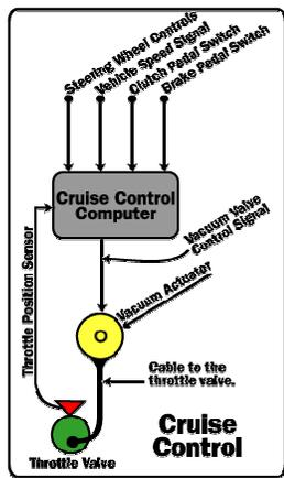
Fig. 3. Working of Cruise Control System
