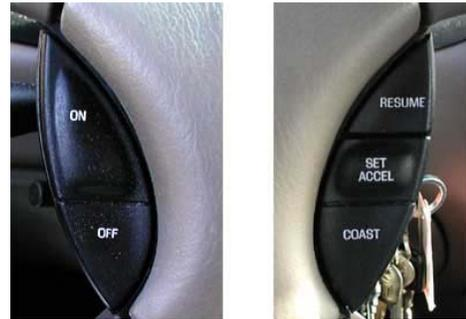
Fig. 1. Cruise Control System Switches on Steering Wheel
